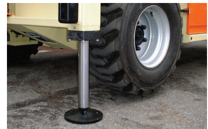
Automatic, self-leveling outrigger system
