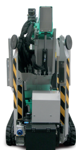
Compact 31" width allows access in narrow, hard to reach places
