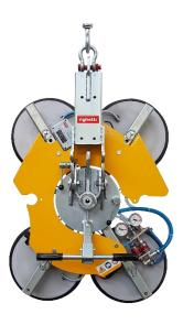
The VB4 d4 is a below-the-hook vacuum lifter suitable for lifting and handling glass units weighing up to 600 kg. Vacuum glass lifter VB4 RCMBM d4 is **battery powered** by rechargeable batteries that, if necessary, may be easily removed and quickly replaced (battery charger included).
