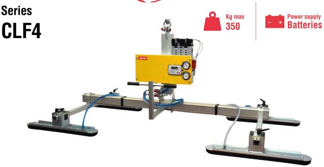
Vacuum lifter CLF4 is the perfect solution for installation of sandwich roof panels. It is equipped with **4 suction** pads (800 x 120 mm), resulting in a maximum lifting capacity of 350kg.
